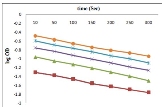
**Figure - 5:** A graph of Log OD versus time (Sec) shows first order with respect to Hexacyanoferrate (III) for Ru (III) catalyzed reaction.
