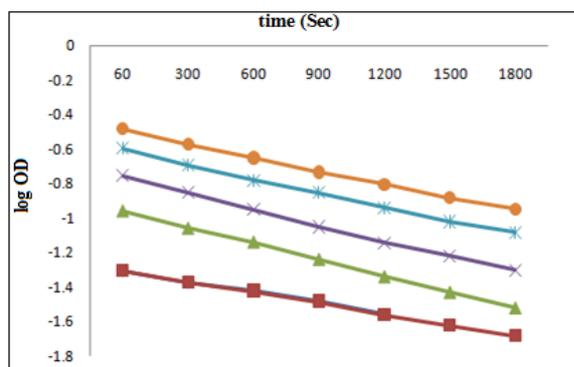
**Figure - 4:** A graph of Log OD versus time (Sec) shows first order with respect to Hexacyanoferrate (III) for uncatalyzed reaction.
