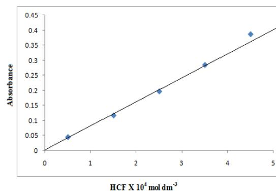
**Figure - 3: Verification of Beer's law for HCF(III) at 420 nm in 0.1 mol dm<sup>-3</sup> NaOH.**
