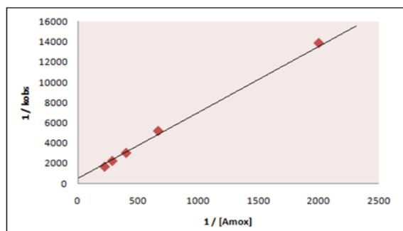
Figure - 8: Plot of 1 / k<sub>obs</sub> versus 1 / [Amox] for uncatalyzed reaction supporting the verification of rate law.
