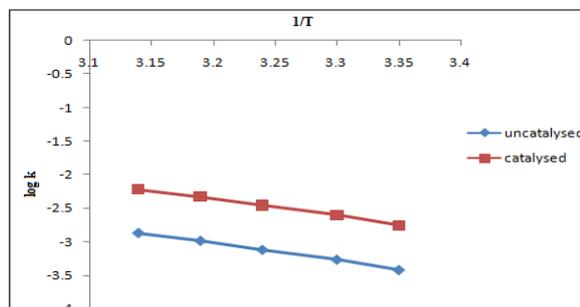
Figure - 9: Arrhenius plot for variation of temperature for Ru (III) catalyzed and uncatalyzed reaction.
