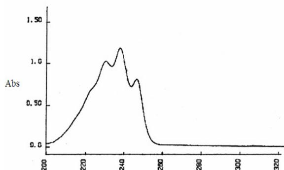
Figure - 4: UV Absorption Spectra of simvastatin.
