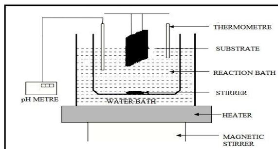
Figure - 1: Experimental set up for CBD.
