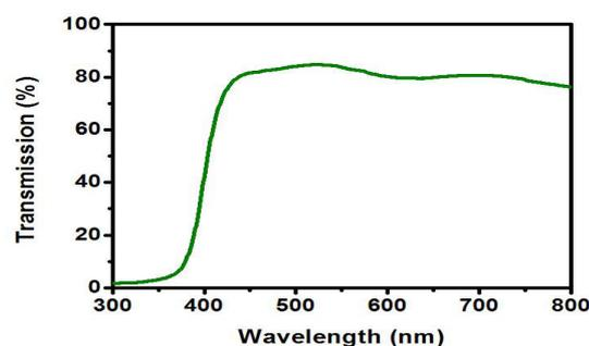
Figure - 4: Transmission spectrum of the  $ZnS$  films.
