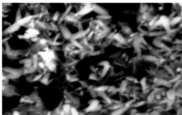
Figure - 3: SEM image of the  $ZnS$  thin film.
