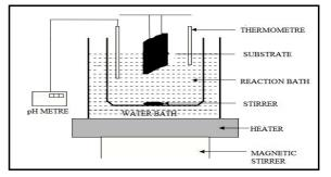
Figure - 1: Experimental set up for CBD.
