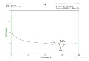
Figure - 5: DSC heating traces of compounds at 1°C/min for the compound 8g.
