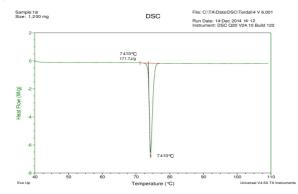
Figure - 2: DSC heating traces of compounds at 1°C/min for the compound 8d.
