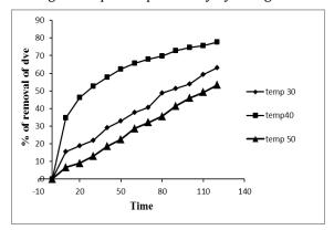
Figure – 5: Outcome of temperature on methylene blue adsorption on activated carbon.
