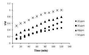
Figure - 8: Pseudo first order adsorption kinetic plots for the adsorption of methylene blue on activated carbon.
