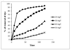
Figure - 4: Effect of dye concentration on % of removal of dye by activated carbon.
