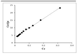
Figure - 7: Langmuir adsorption isotherm for adsorption of methylene blue on Activated carbon.
