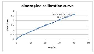
Figure - 2: Calibration curve of olanzapine.
