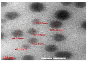
Figure - 6: Droplet sizes of NE formulation are determination by TEM.
